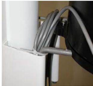
2. Mount the support tube as indicated; A tripod is shown. You can also use U-bolts or a Mono Mount. Insert the neck down end into the **MKIII** sensor assembly until it bottoms with the retaining screw in the slot. Tighten the screw.
