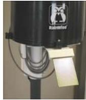
This leaf wetness sensor is designed to be mounted on the North side of the MK-III weather station. The bracket provided with the sensor insures a solid and secure installation.
